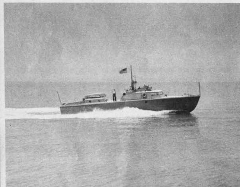
Shore-based 63-ft. boat can rush casualties in from open sea at more than 30 knots, while shallow draft permits speedy navigation of coastal waters near bases. It has low streamlined cabin, enclosed hatchway aft.
